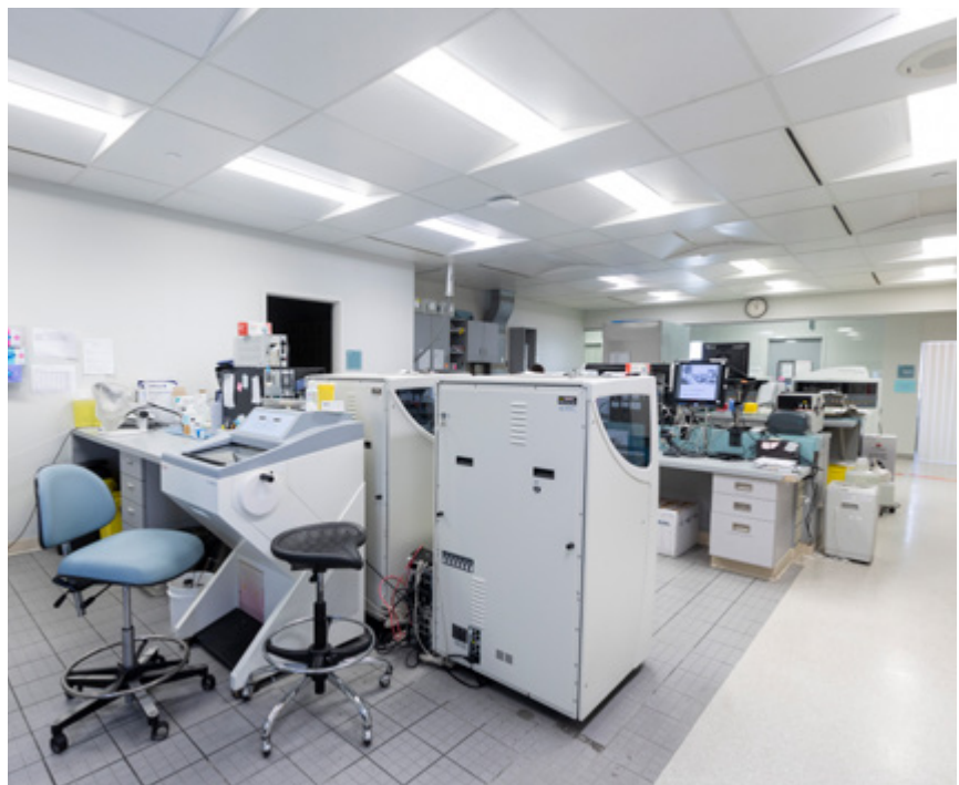
Immunohistochemistry Cryostat: Fresh tissue (Kidney, skin and muscle biopsies) cut at -23 degrees in order to prepare slides for Immunohistochemistry tests.
