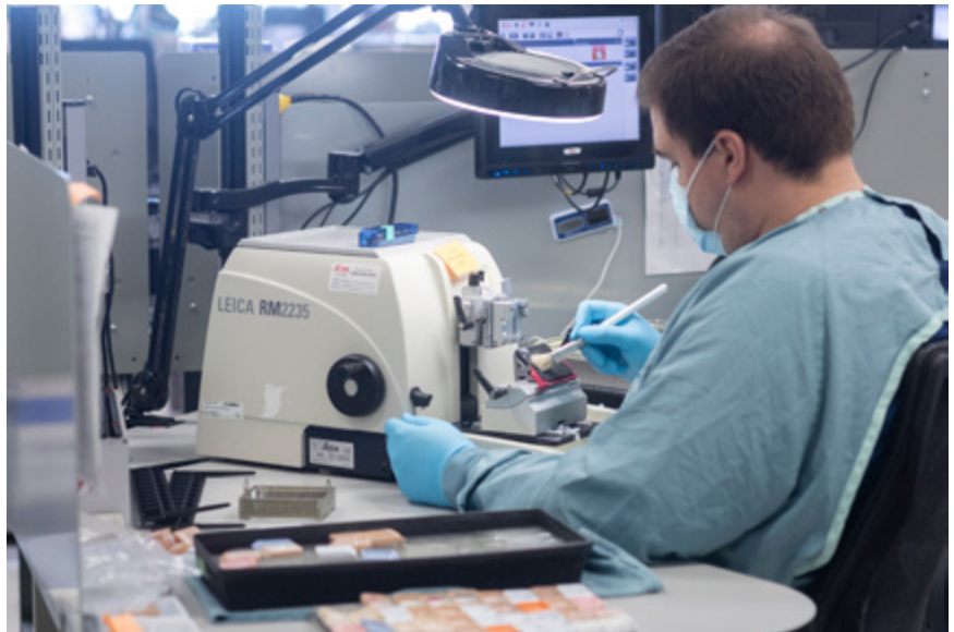
Evan Nault: Performing microtomy of a wax block after embedding.
