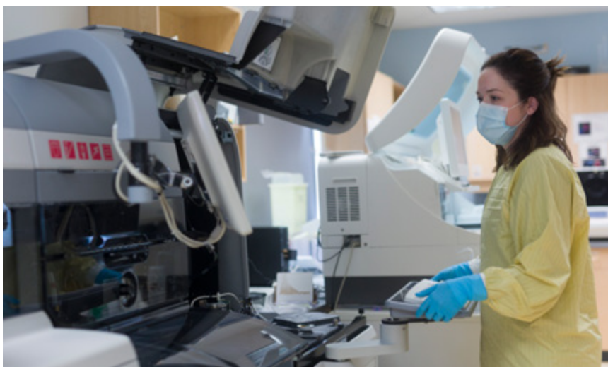
Megan Dallyn – Performing Maintenance on the Vitros 5600 Chemistry/Immunoassay Analyzer
