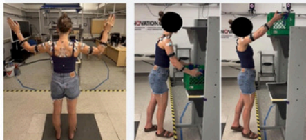
Figure 1: Motion capture marker and EMG sensor placement (left) and overhead lifting task (middle, right).
